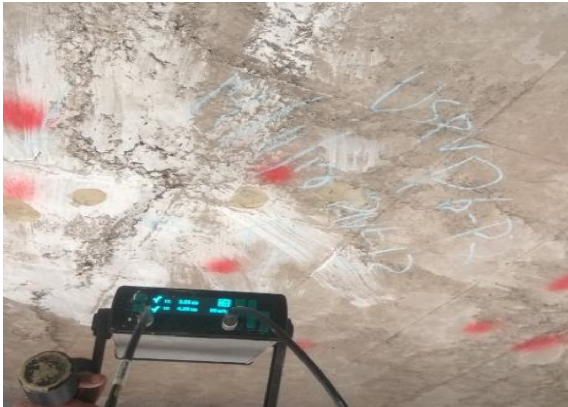
Photo 77. Crack pattern analysis using the USPV
