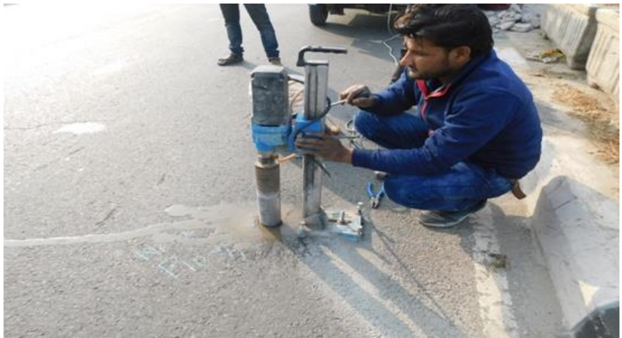
Photo 75.Core sample is being extracted for compression test
