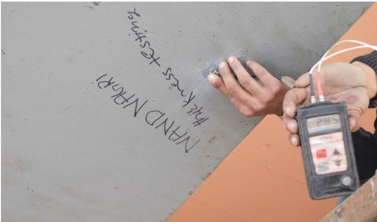
Photo 79. Thickness Testing on steel with Ultrasonic thickness gauge
