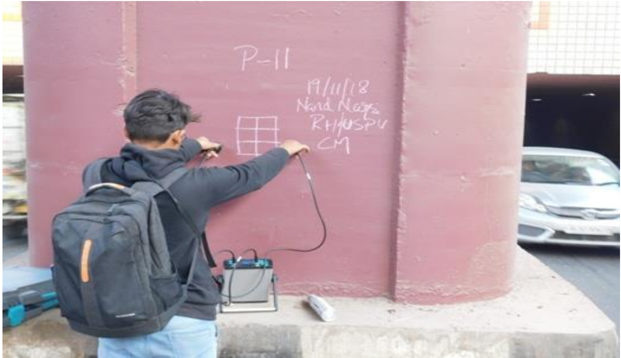
Photo 72.USPV Test on Pier P11
