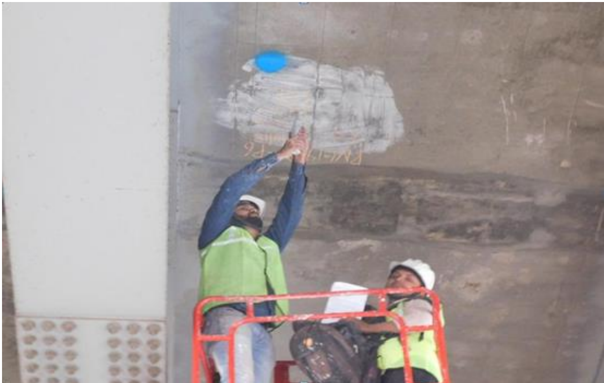
Photo 71. Rebound hammer Test on Panel
