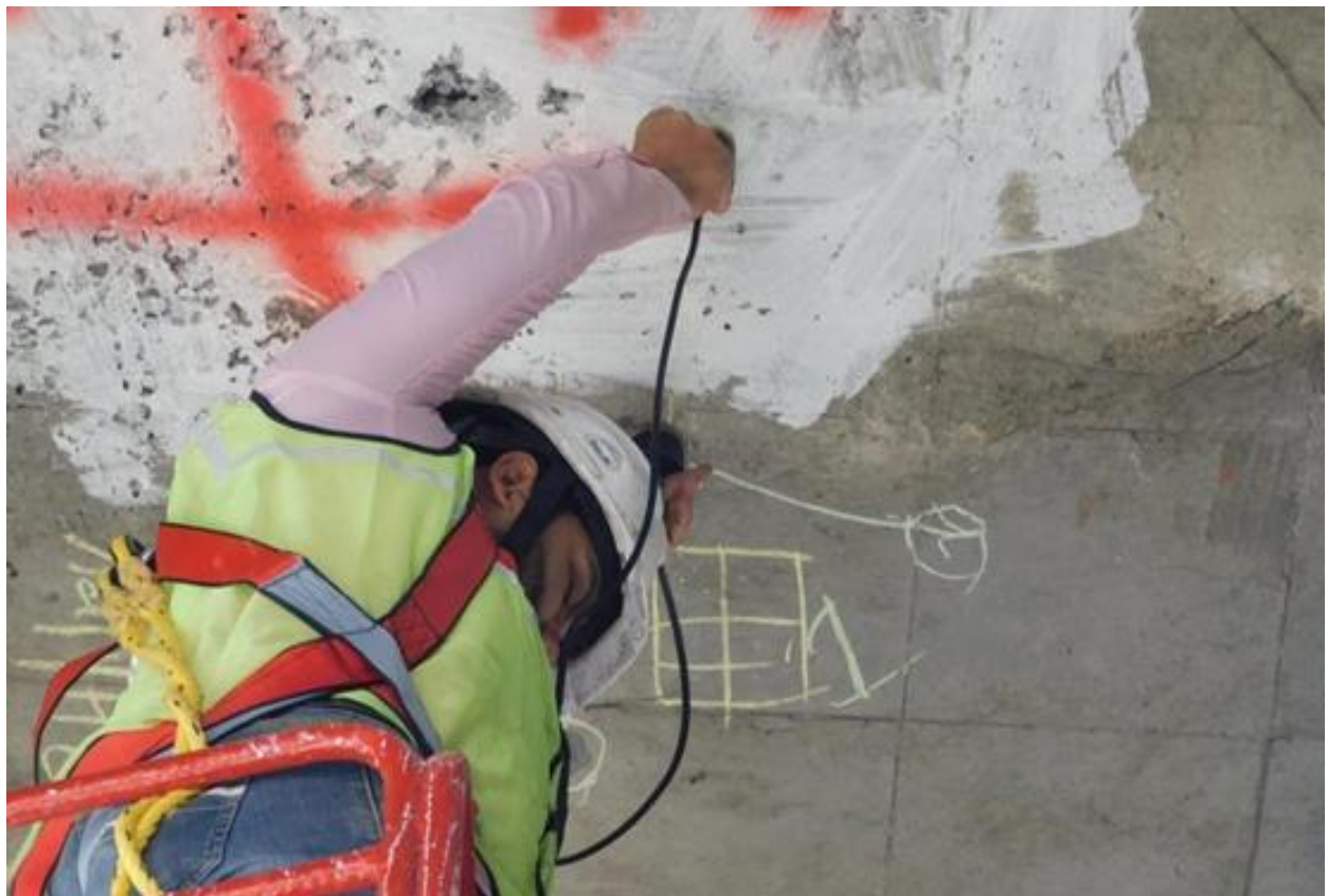
Photo 73.USPV Test on Panel
