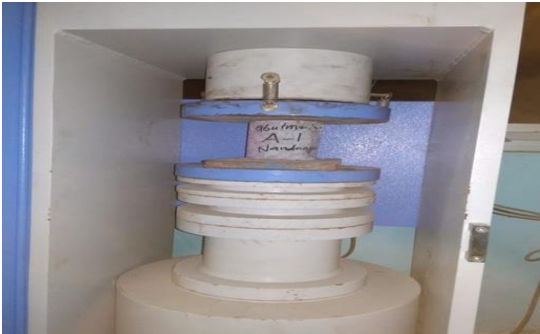
Photo 76. The core sample is placed and tested using Compression Testing Machine
