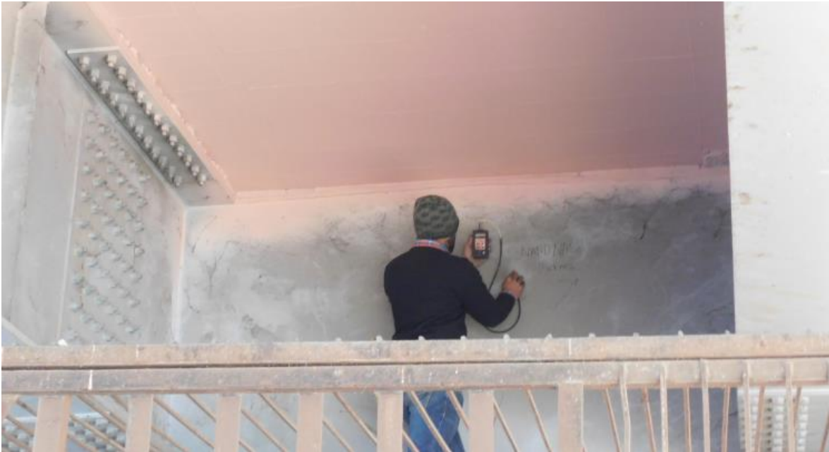
Photo 78. Thickness Testing on steel girders and diaphragms
