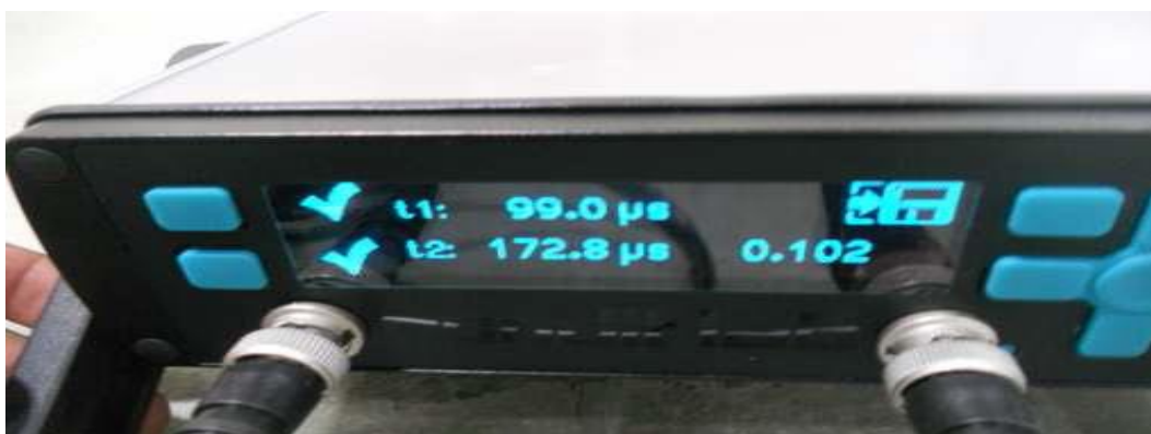
Photo 62. UPV meter showing T1 and T2 readings
